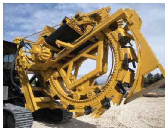
Heavy Duty Heat Treated Buckets and Drop Forged Teeth
