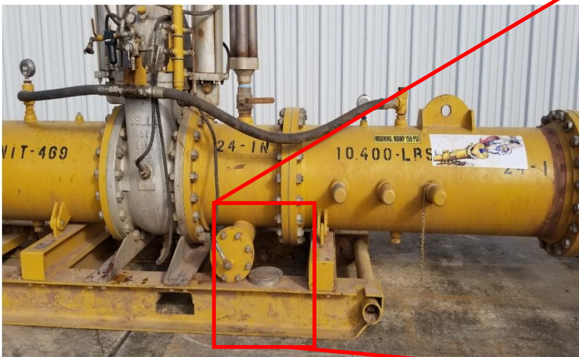
Photos: Launcher shipped with 28lbs. Blind Flange unsecured on the skid.
