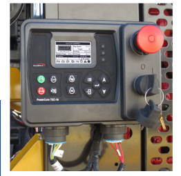
Operator's Control Station
